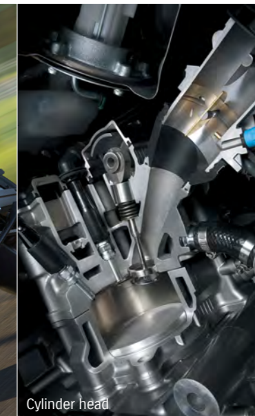
1037cm 3 DOHC, 90-degree V-twin engine
